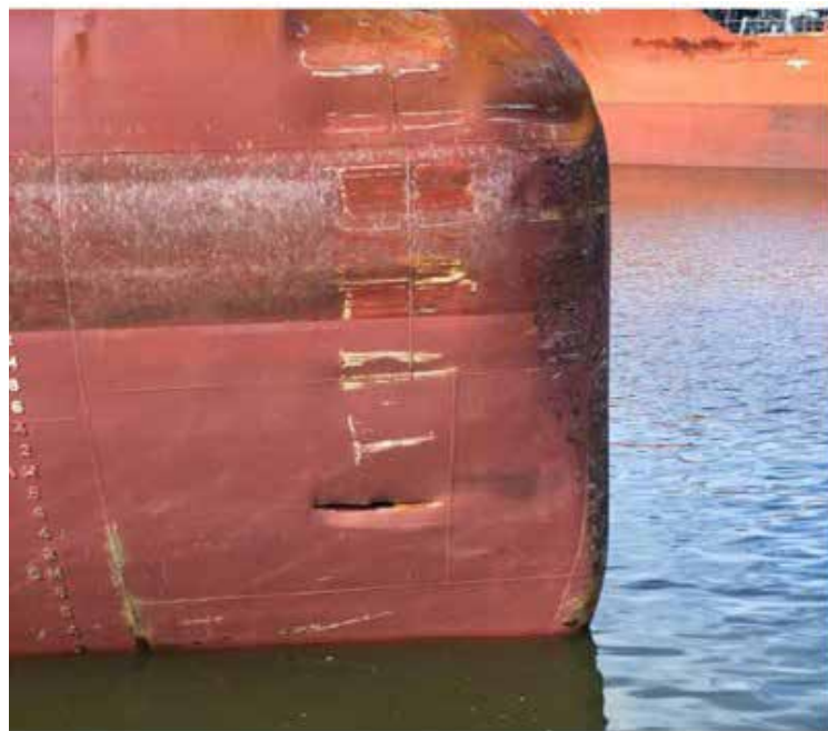
Yochow 's bow showing, at left, holed bulbous bow and depth of penetration and, at right, damaged upper starboard bow.
