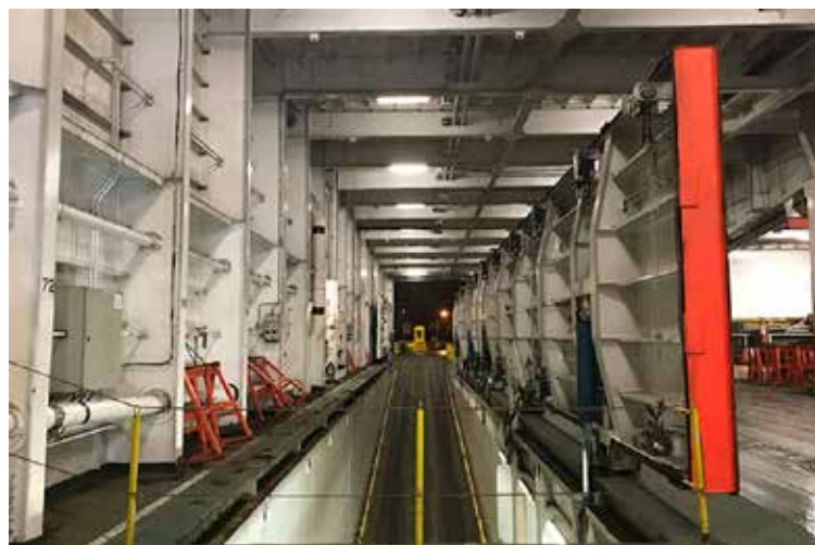
In mv Seatruck Pace the orange-painted leading edge of the open ramp hatch cover is clearly shown.
