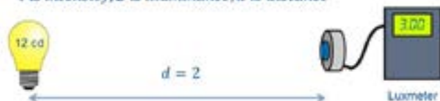
Figure 1 - Measuring intensity with a luxmeter using the inverse square law method
