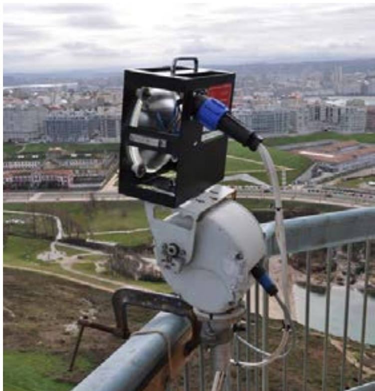
Figure 8 – Reference light and pan and tilt head temporarily installed at the lighthouse
