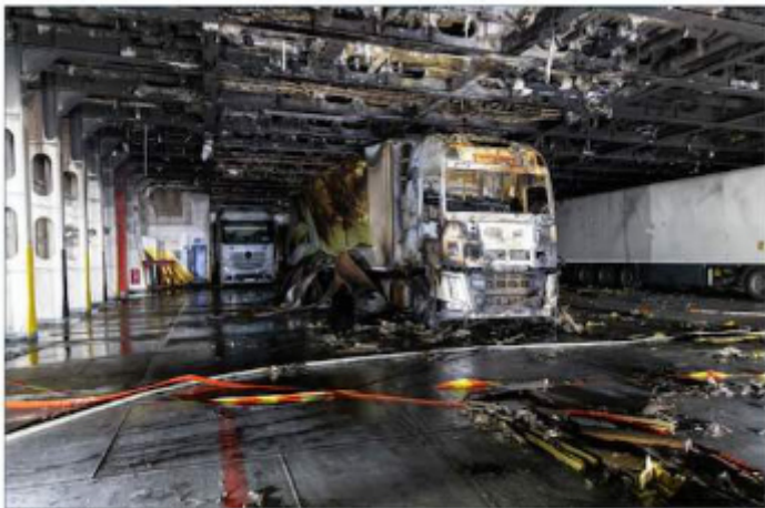
Figure 12: Fire scene on Deck 4.
