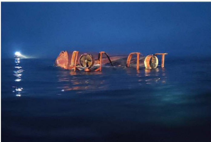
Karin Høj's upturned hull, showing azimuth drive units at the stern.
