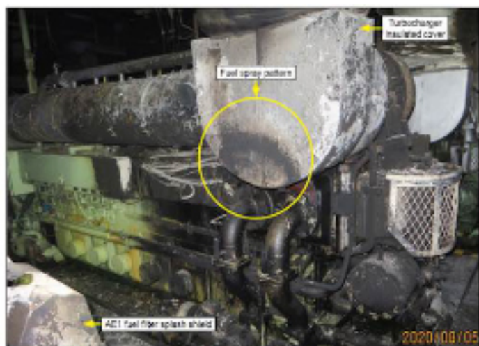
Figure 3: Post-fire AE1 fuel filter splash shield and AE2 turbocharger insulated cover
