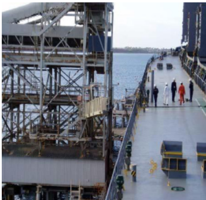
Shore supplied access arrangements.
