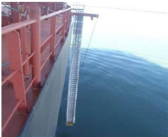
Suspended accommodation ladder.
