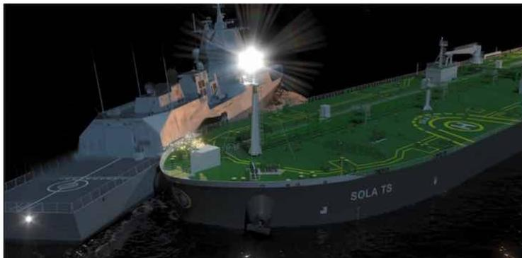
Figure 1: The point of impact when HNoMS Helge Ingstad and Sola TS collided outside the Sture Terminal in the Hjeltefjord at 04:01:15. Illustration: AIBN
