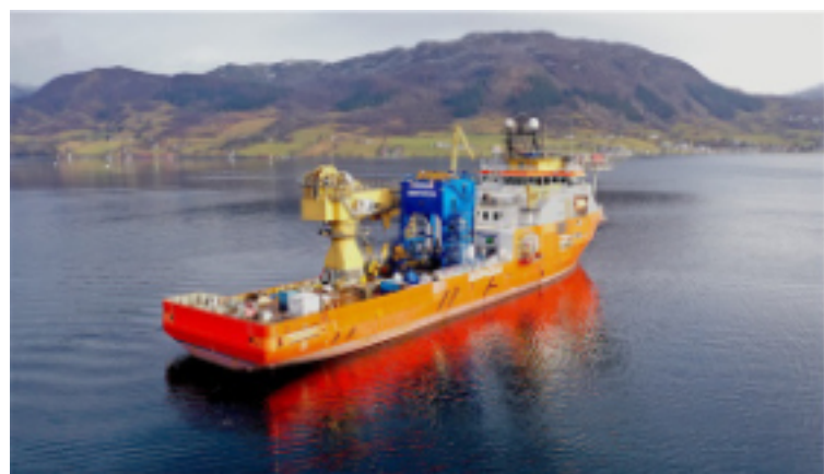
The 6,000-dt CSV Normand Ocean (built 2014) is the latest Solstad Offshore vessel to have been through a diesel-electric retrofit, delivering as much as 25% fuel savings in field and mobilisation/demobilisation operations, and 20% in DP2 mode.
