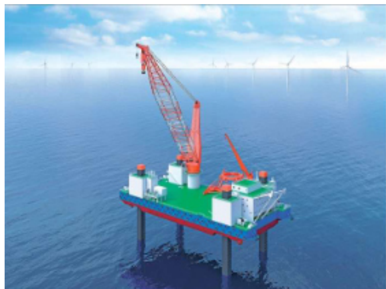
Image of the self-elevating platform vessel. Courtesy of Toa Corporation.
