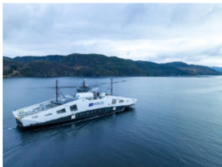
Hydra with the white hydrogen tank visible.
