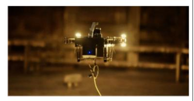
It is understood that the DNV-led project is testing drone technology, developed by Scout Drone Inspection that are capable of navigating in confined spaces, such as cargo tanks. This provides valuable input and requirements from the owner's perspective for future drone tank surveys. DNV recently adapted their survey process for the use of drones and implemented supporting software.
