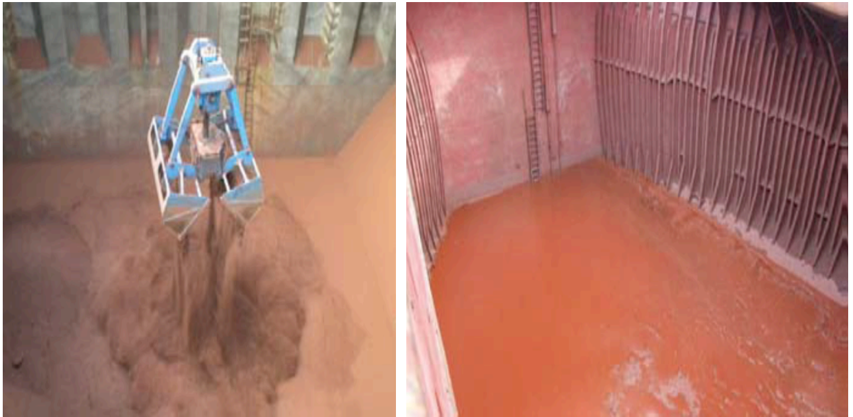
Fig 2: Iron ore fines before and after liquefaction [12]
