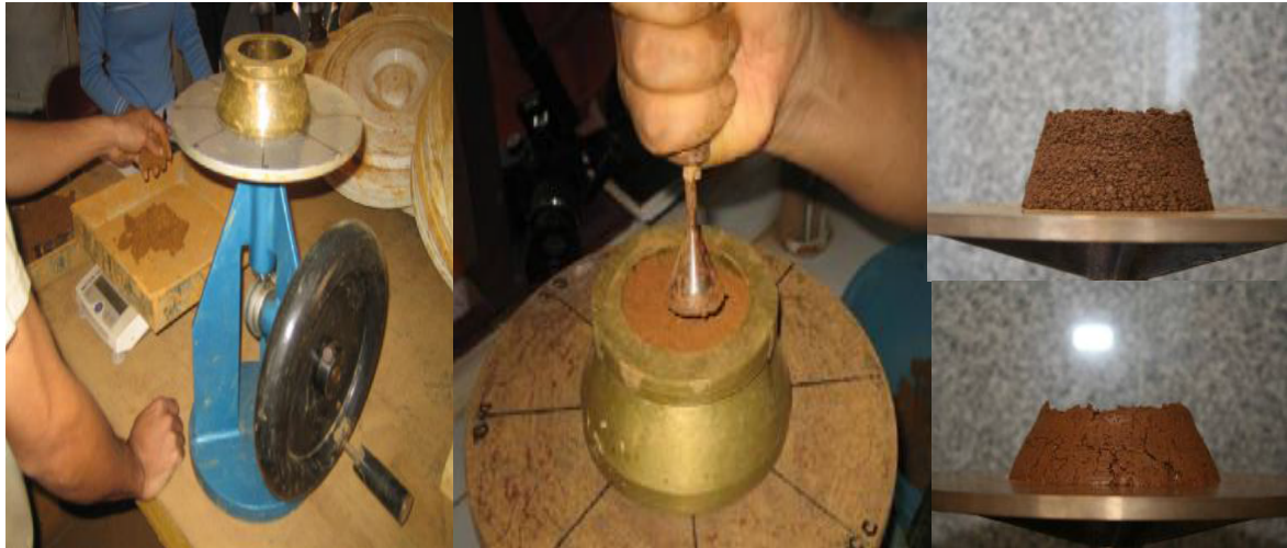
Fig 4: Flow Table Test [9].
